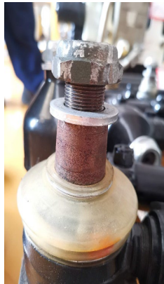
Figure 1: Corroded component from an underbody system of an armored combat vehicle.
