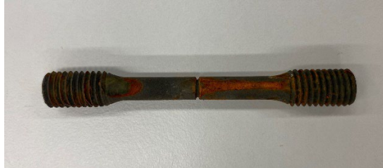
Figure 9: Zinc-phosphate coated AISI 4340 specimen after 24 hour salt spray test.
