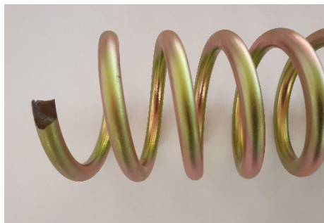
Figure 2: A fractured spring of a component due to hydrogen embrittlement.
